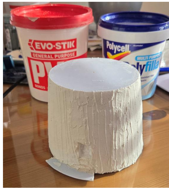
The trimmed polystyrene, and tower coated in Polyfilla
