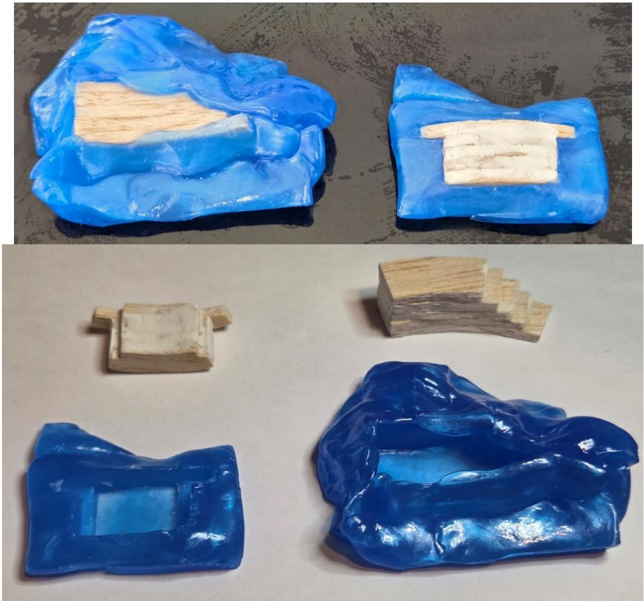
Balsa masters forming the Blue Stuff moulds
